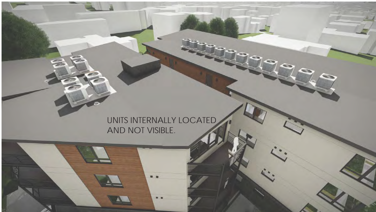
FOR MORE INFORMATION, SEE ROOF PLAN, SHEET A1.5. MECHANICAL EQUIPMENT WILL NOT BE VISIBLE FROM PEDESTRIAN PERSPECTIVE
