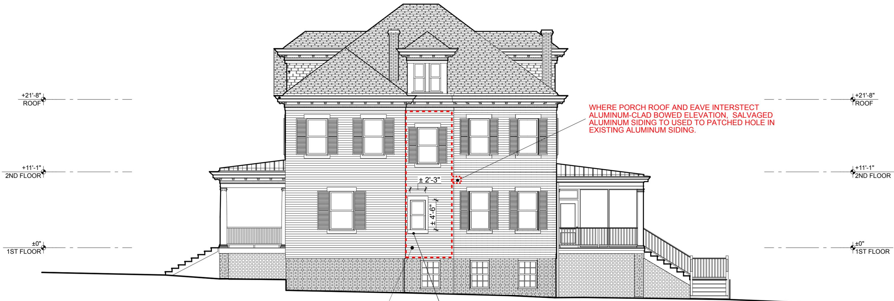
WHERE PORCH ROOF AND EAVE INTERSECT ALUMINUM-CLAD BOWED ELEVATION, SALVAGED ALUMINUM SIDING TO BE USED TO PATCHED HOLE IN EXISTING ALUMINUM SIDING.
