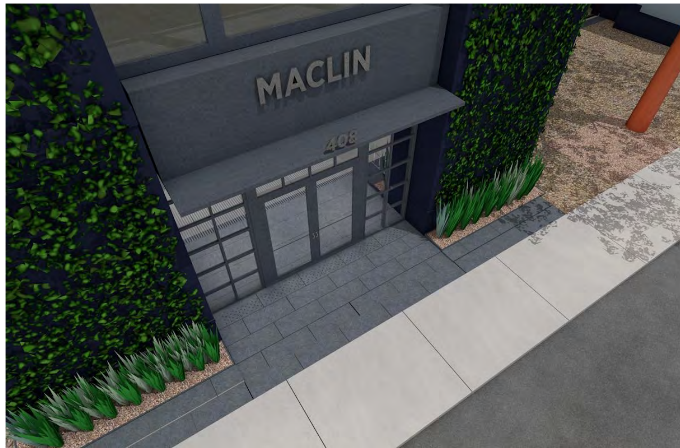
BLUESTONE PAVER LAYOUT BASED ON 12X36 AND 15X48 LANDSCAPE TREADS (NO CHANGE TO COURTYARD SURFACE PROPOSED). DEPTH OF PLANTERS FLANKING ENTRY IS APPROX. 24", HALF THAT OF THE EXISTING RAISED PLANTERS.
