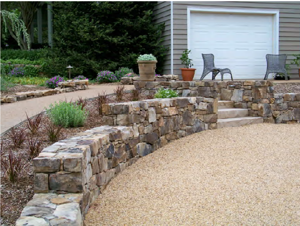
Proposed Fieldstone Retaining Walls and Free-Standing Walls: All proposed walls to be CMU block walls with fieldstone veneer in a dry-laid appearance laying style with raked joints. The proposed walls to have the same appearance as the above precedent images.
