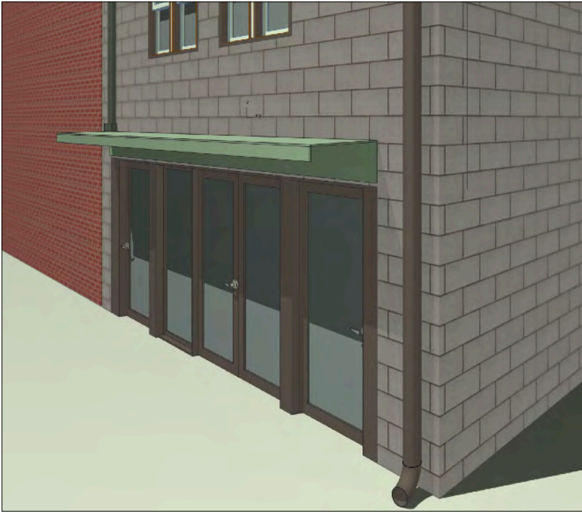
AWNING- BENT METAL, BOLT TO WALL
