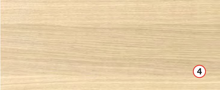
White Oak (multi-coat clear finish) at exterior soffits and back of stair recess
