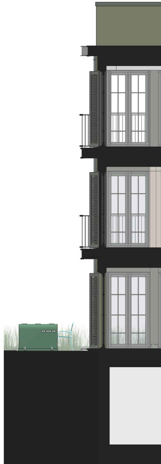
condition B section at door(s) with balcony depth of balcony typically less than 1'-8" (exception: balcony at SE corner)
