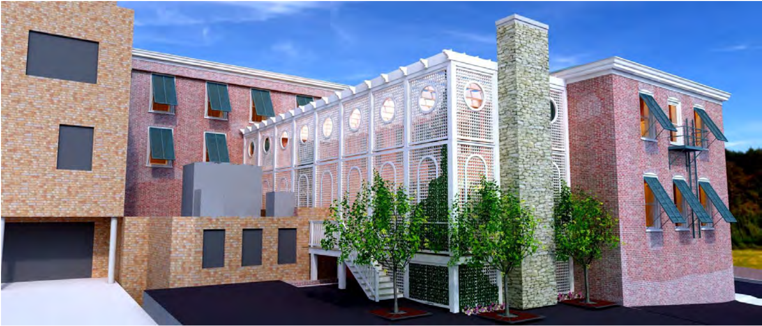
PHOTO 26 – DECK WITH ARBOR AND TRELLIS TO BE BUILT TO OBSURE SATELLITE DISHES AND AC CHILLER
