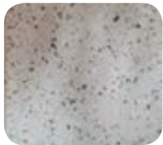
P.I.P. CONCRETE EXPOSED AGGREGATE 6" Curb, Flex Zone, and Driveway Aprons
