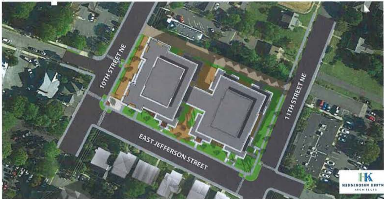
Site Plan showing increased setbacks, pedestrian plazas, streetscape improvements and on-site alley.
