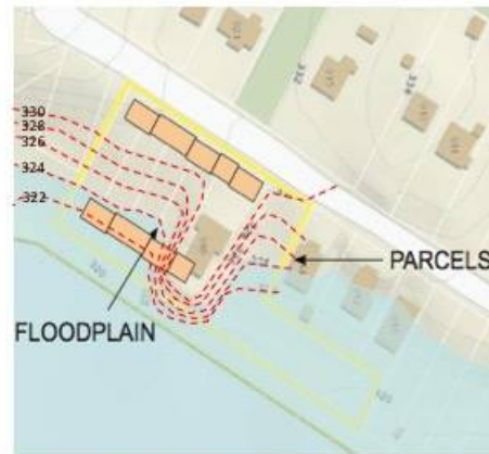
Accurate Floodplain Map (approved 2.6.2017) Floodplain per field survey and current floodplain study.
