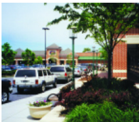
In this commercial development, smaller pedestrian-scaled light fixtures are placed along the sidewalk while a taller non-decorative light fixture is used for general lighting in the parking areas.
