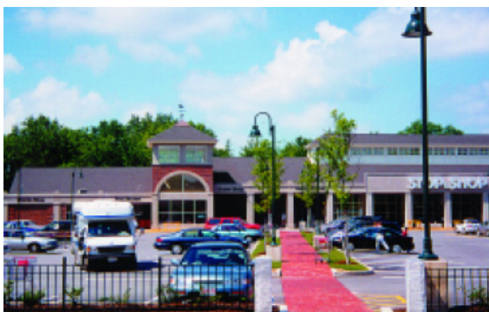
This brick sidewalk connects a public sidewalk with the deeply setback commercial development. Note the trees and light fixtures lining the walk and the brick crosswalk. The walk is aligned to minimize its visible impact on building features and storefronts. Lastly, note the metal fence, granite piers and planting strip that define the front edge of the development.
