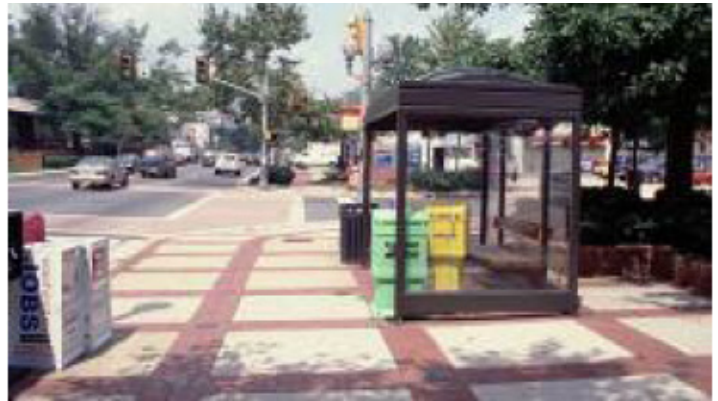
Paving patterns and delineated crosswalks provide pedestrians with a well-defined, inviting pathway along this busy corridor.
