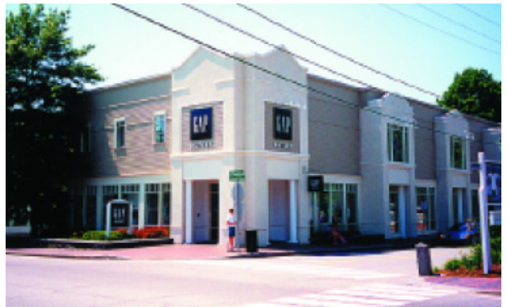
This new commercial building is placed at the intersection with minimum setbacks to help define the corner.
