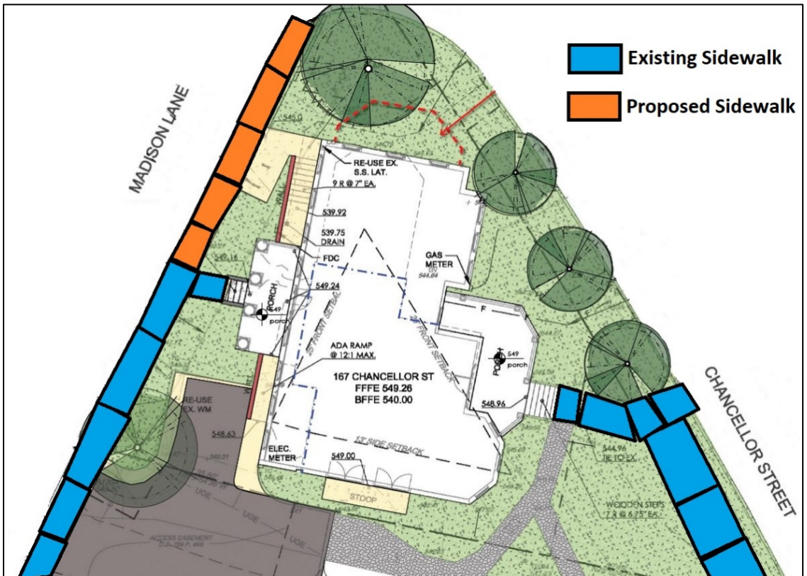
Diagram of existing and proposed sidewalk. - SOURCE: Applicant Preliminary Site Plan and SUP applications (09/17/2019)
