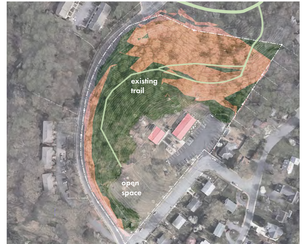
EXISTING SITE DIAGRAM SHOWING WOODED AREAS WITH CRITICAL SLOPES (ORANGE) AND WITHOUT CRITICAL SLOPES (GREEN) EXISTING TRAILS SHOWN IN LIGHT GREEN LINWORK
