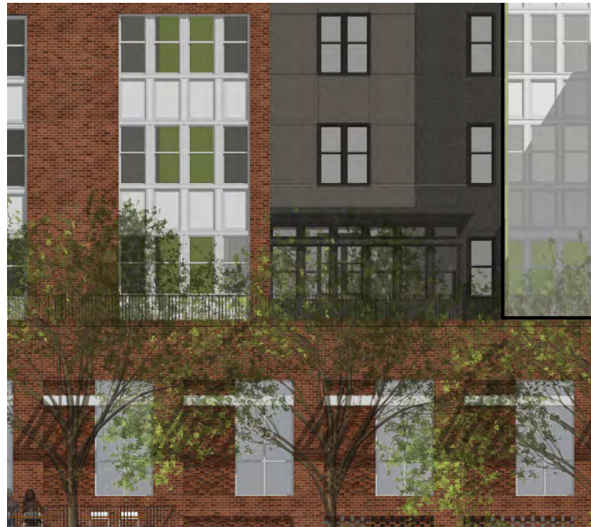
Windows and doors are all vertically proportioned
